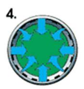
The vessel is pressurised forcing the preservative into the timber.
